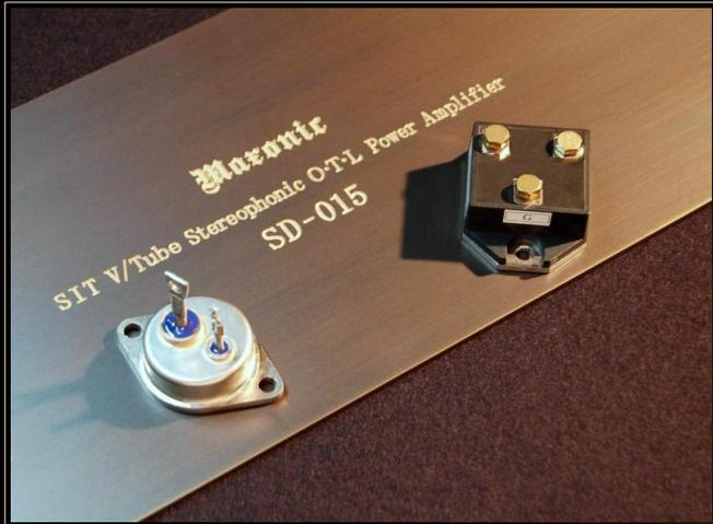
The sole, pure Japan-born semi-conductor developed by Dr. J. Nishizawa, ex-president of Tohoku University and world-known authority of metal engineering which utilises induction effects of statics makes it possible to treat large current under low electricity consumption : Its reduction capability of channel resistance to the absolute minimum assures low inner resistance, high speed and low energy loss, thus realising signal amplification totally faithful to signal wave-forms.
